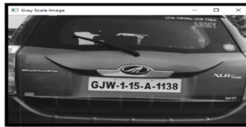
Figure 3: Image converted to gray scale from colour image
