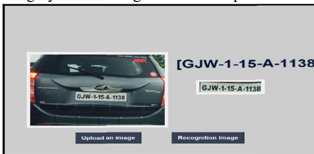
Figure 9: Number plate and characters have been recognised and
