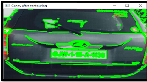
Figure 5 (a): Contours Based on Image
